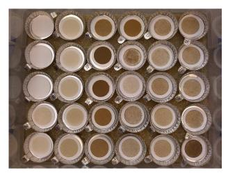
All water samples are vacuum filtered through quartz fibre filter (QFF) papers to extract the suspended solids. Source area sediments are also transferred onto QFF papers after being wet sieved to 63 µm to extract the fine silts and clays that become suspended in-stream. These filter papers are subsequently analysed by both **XRFS** and **DRIFTS** to determine the concentrations of major elements and compounds.
